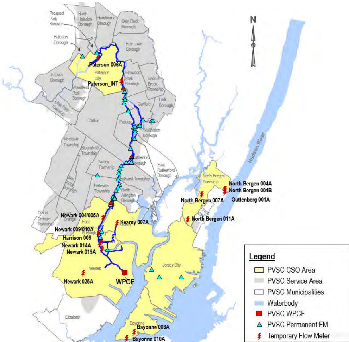
Figure E-1 shows the locations of the flow meters, including both permanent and temporary flow meters, which were used for H&H Model calibration and validation.
