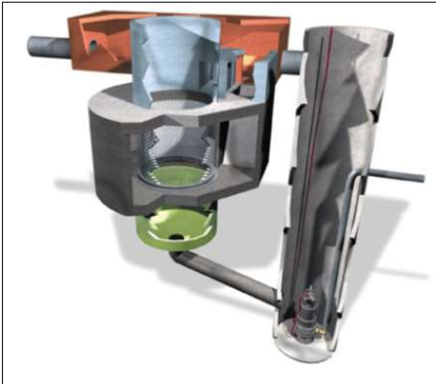
Figure 2-11 - Cross Section of a SanSep Unit
