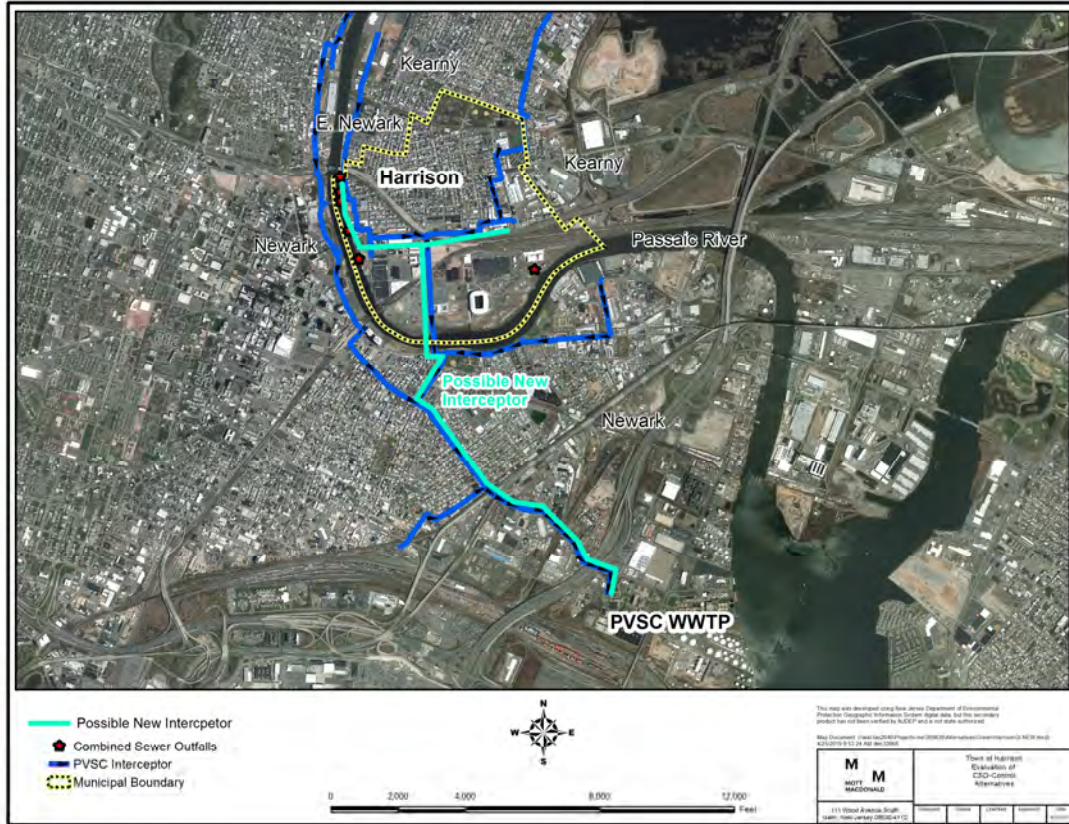
Figure 13: Conceptual conveyance conduit route from Harrison to PVSC
