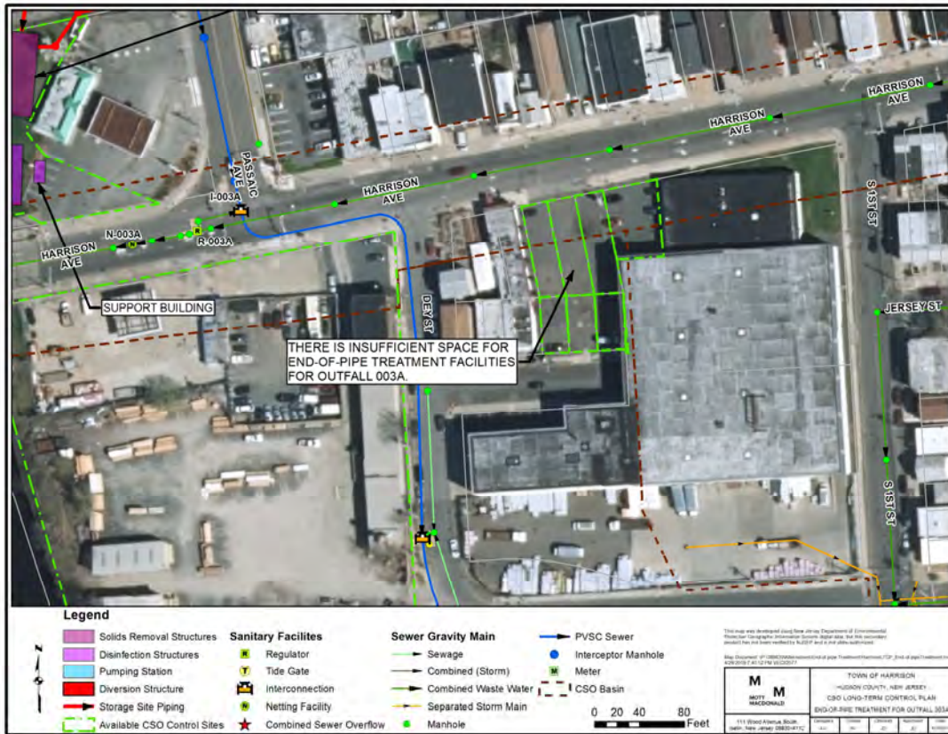
Figure 45: Point Treatment - Outfall 003A insufficient space
