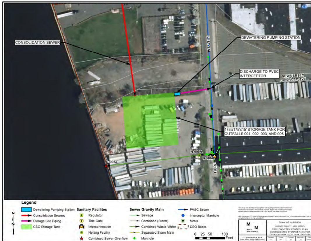
Figure 39: Consolidate Storage - Storage Tank
