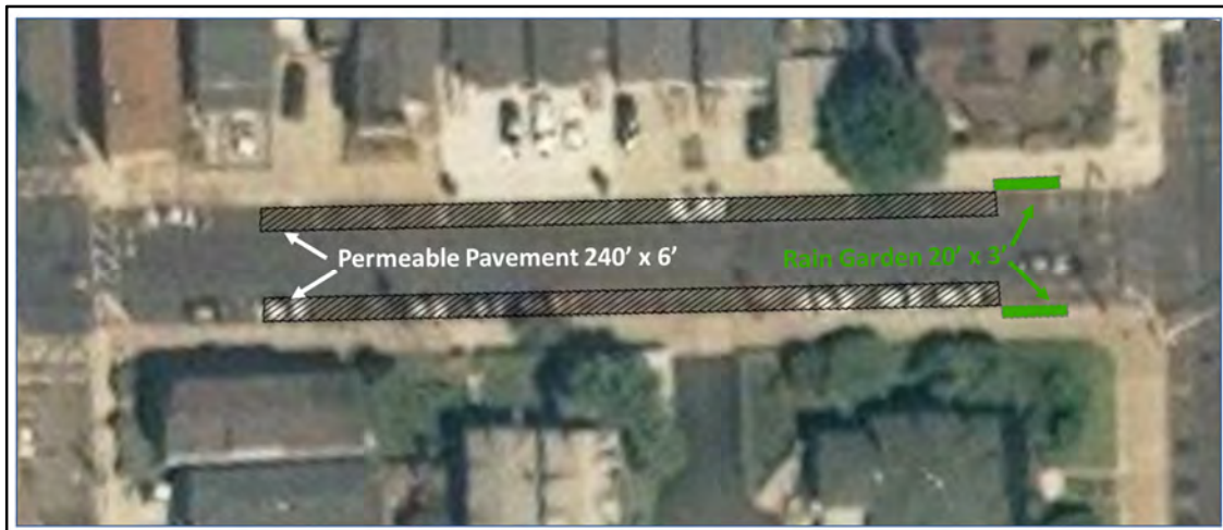
Figure 53: Typical street segment with green stormwater infrastructure
