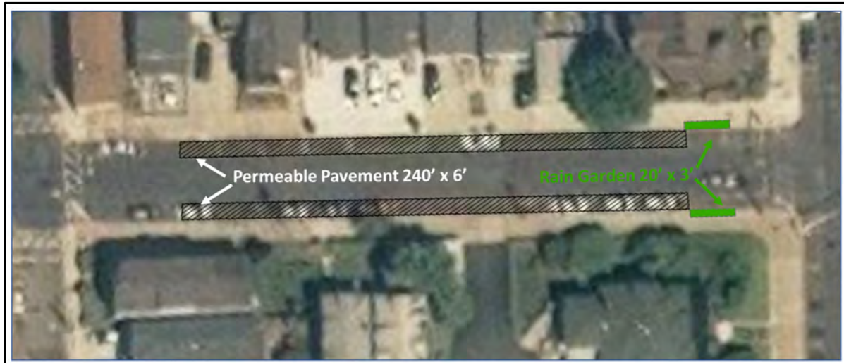
Figure C-15: Typical street segment with green stormwater infrastructure
