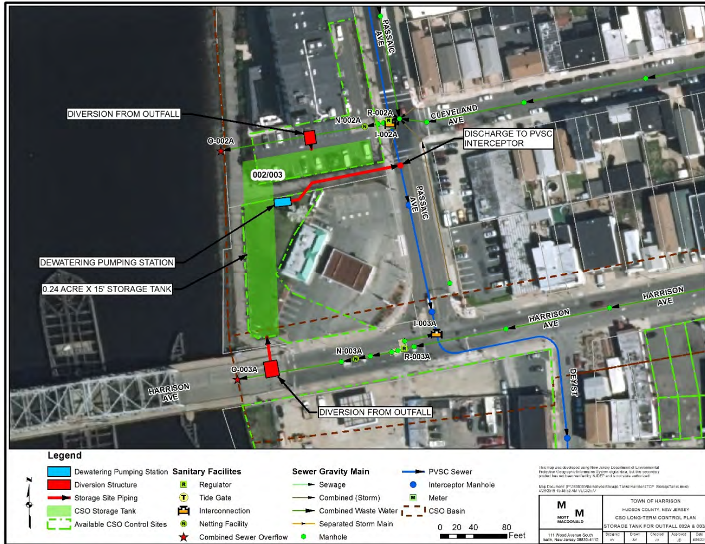
Figure C-2: Point Storage - Outfall 002A and 003A (Site 002A/003A)
