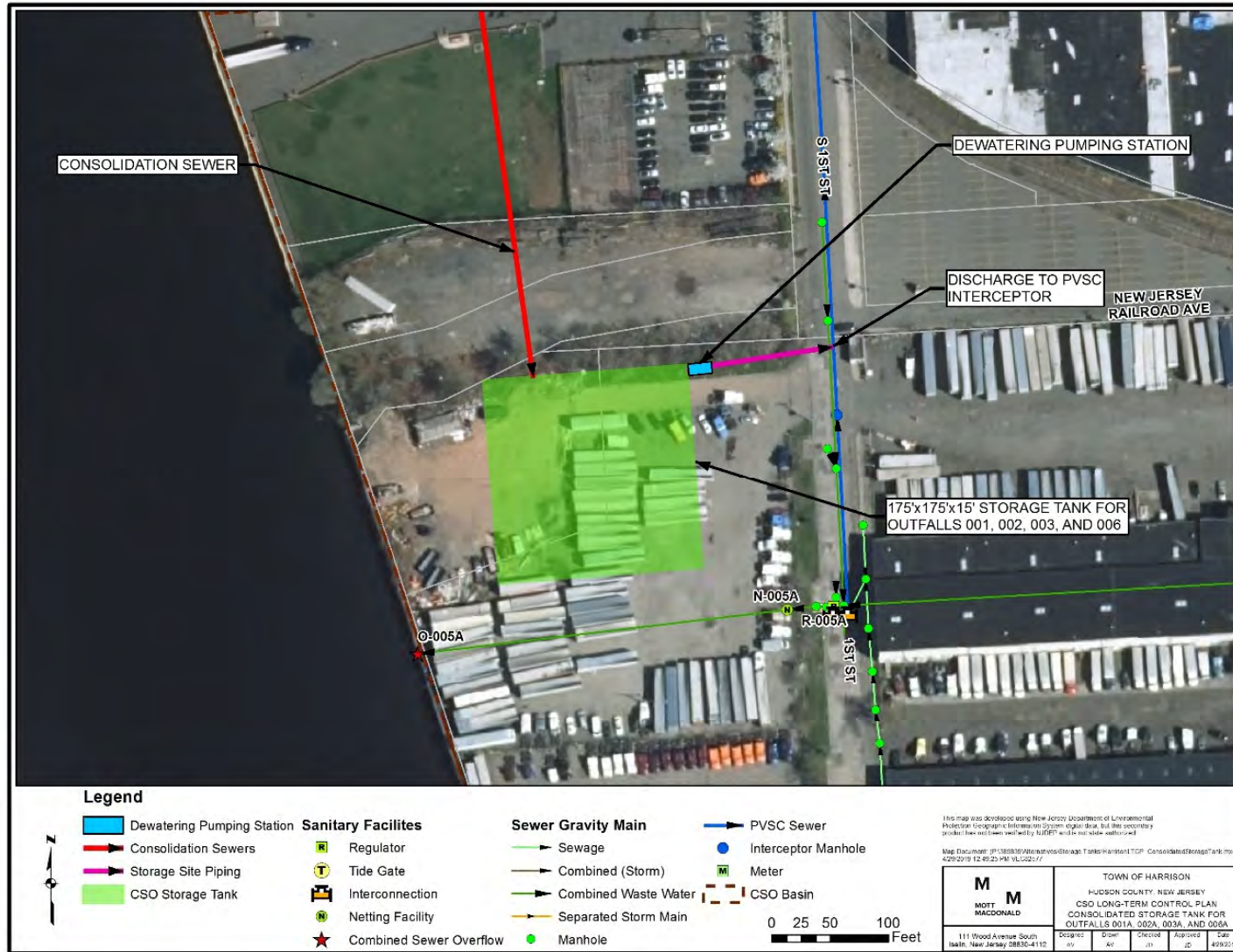
Figure C-6: Consolidated Storage Tank for Outfalls 001A, 002A, 003A and 006A
