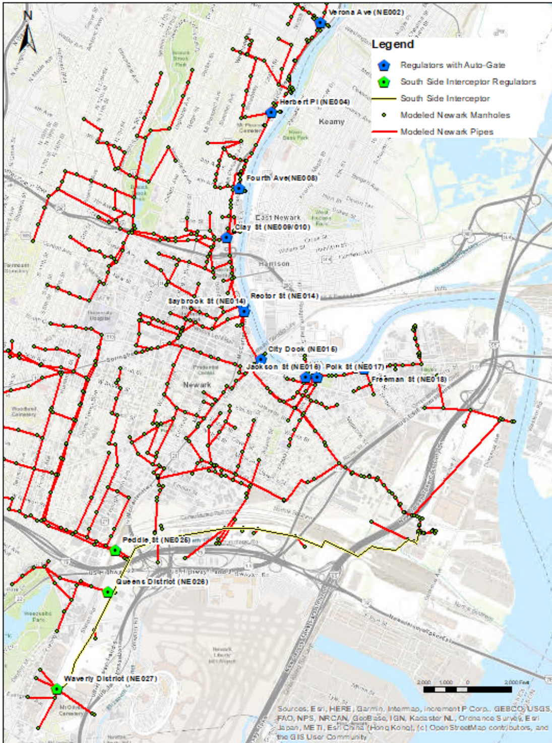
Figure D-5. Newark Regulators with Automated Controls and South Side Interceptor Regulators
