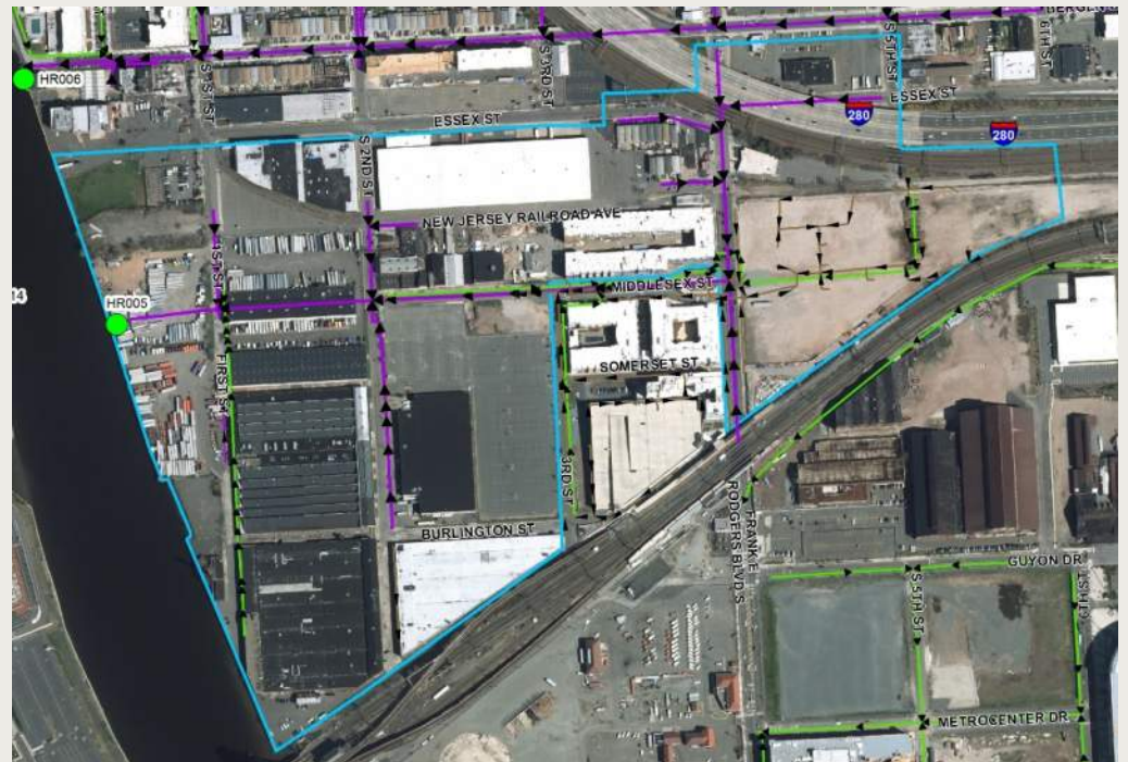
Drainage Area and Sewers for CSO 005
