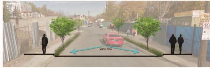
A section perspective of Presidential Boulevard in Paterson New Jersey. These 2 foot wide "Green Gutters" can be implemented on more narrow streets to maximize the storm water retention within a small area
