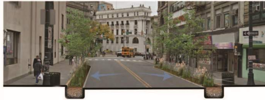
A section perspective of Market Street in Paterson New Jersey. These 6 foot wide "Roadside Bioswales" can be implemented on medium to large streets to hold and retain stormwater runoff and lessen the amount of rainwater that ends up in Combined Sewer Systems
