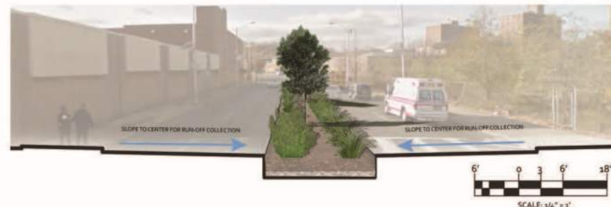
Memorial Drive is a 79 foot wide four-lane road. A long stretch of 15 foot yellow line dividers serve as optimal location for a bio-swale divider to collect and clean run-off. Areas where turning lanes exist could have metal grates to continue the water storage swale.
